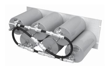
The Telewave TPRD-4546 UHF Duplexer allows simultaneous operation of a transmitter or combiner and receiver into a common antenna. This band-pass/band-reject duplexer provides maximum TX-to-RX isolation with minimum insertion loss. Six 4" high "Q" cavities in a pass/reject configuration provide better isolation with close frequency spacing than an equivalent bandpass-only duplexer.
