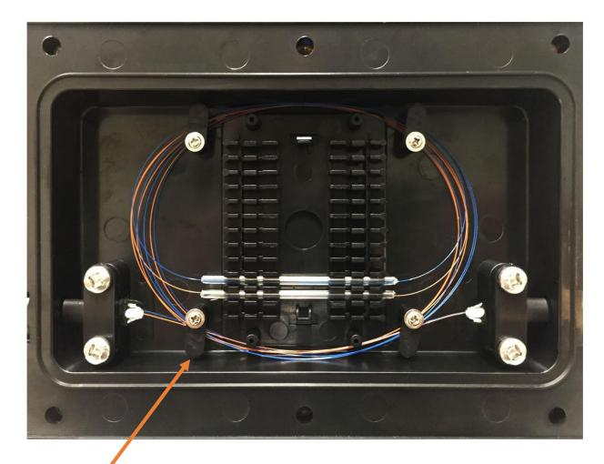
The four fiber retention wings are positioned to keep the fibers captive to the base of the DFE100 so the fibers do not fall or spring out of position.
