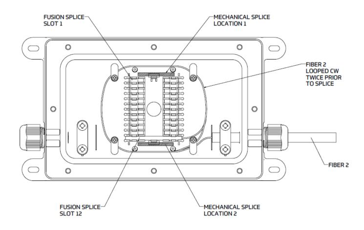
The picture below shows the DFE100 with two fibers loaded into the splice tray as would be typical with a FTTH drop fiber repair. The orange fiber on the left-hand side routed counterclockwise and the orange fiber on the right-hand side routes clockwise so that the splice protector mounts in splice #11 position.
