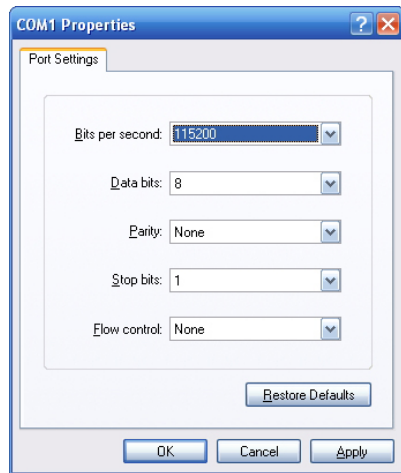
Figure 3-2: COM Port Configuration
