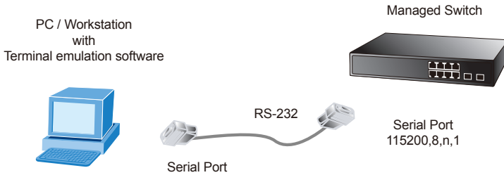
Figure 3-1: Managed Switch Console Connectivity
