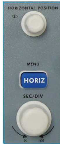
Fig. 3-12 Horizontal Control Zone
